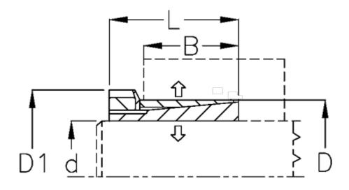
$\begin{array}{lll} \text{B mm} & = 22 \\ \text{D1 mm} & = 45 \\ \text{d H8 mm} & = 25 \\ \text{D mm} & = 35 \\ \text{Fit tolerance} & = \text{Aksel h8, Nav H8} \\ \text{F kN torque} & = 20 \\ \text{L mm} & = 35 \\ \text{P N/mm2 surface pressure on shaft/hub} = 60 \\ \end{array}$
